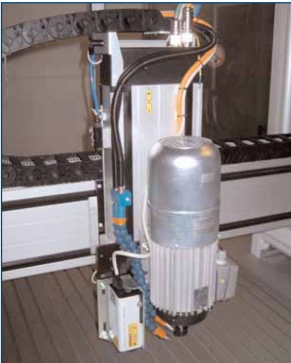
Kombination CONOPROBE-Laser und MAW 2.22-K / combination of CONOPROBE laser and MAW 2.22-K spindle motor
