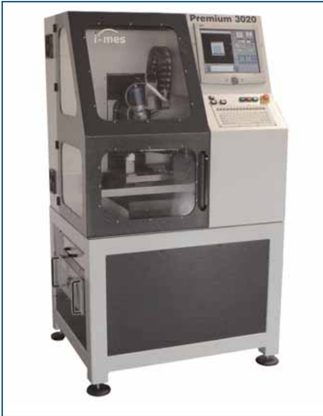
PREMIUM 3020 mit 4-/ 5-Achse / PREMIUM 3020 with 4th / 5th axis
