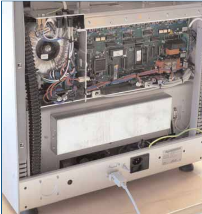
IMC4-Steuerung eingebaut in der Maschinenserie ICP / IMC4 controller mounted in the machine series ICP
